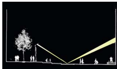
The rhythmic patterns on the surface of the water are reflected on to the large town hall façade by cleverly devised lighting management.
