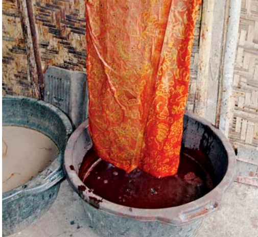
The fabric with the wax design is repeatedly dipped into the dye
